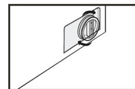
**Warning!** Never remove the pump cover when the washing machine is in operation, always wait until the appliance has finished and it is empty. There can be hot water within the pump, so be careful to avoid burns, should it have operated recently. When replacing the cover, be careful to ensure it is closed securely.
